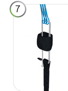
7 Push the looped end downward through the elastic sleeve (not small diameter tube) first, and then through the loop with the reinforced end (black tab) once more.
