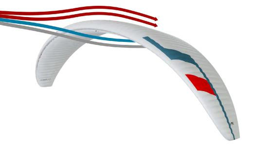
Let go of the lines to re-inflate the tips automatically. If they do not, try progressively pulling one brake then the other. Asymmetric reopening is recommended in order to avoid compromising the angle of attack, particularly flying near the ground or in turbulent conditions.
