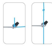
Diagram 1. Speed-bar connection by means of Kite loop (without Brummel hook)
