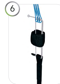
6 Push the looped end first upward through the elastic sleeve (not small diameter tube) and through the lines again following the same pattern.
