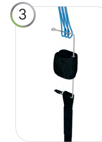
3 Push now the IKS line through the lines and the riser. The reinforced end with the black tab should be located on the riser side.
