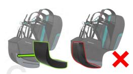
Insert the foam and position it correctly.
