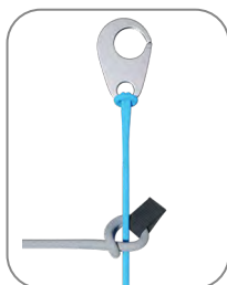
Diagram 2. Speed-bar connection by means of kite loop (without Brummel hook).
