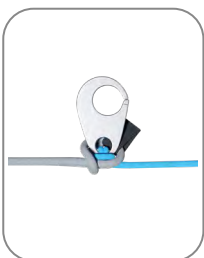
Diagram 1. Speed-bar connection by means of the Brummel hook.
