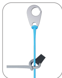
Diagram 2. Speed-bar connection by means of kite loop (without Brummel hook).
