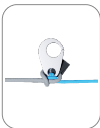
Diagram 1. Speed-bar connection by means of the Brummel hook . The blue line is from the harness, and the gray from the riser.
