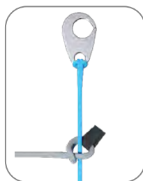
Diagram 2. Speed-bar connection by means of kite loop (without Brummel hook). The blue line is from the harness, and the gray from the riser.
