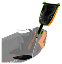
Fill the Infbag with air, close it, and connect it to the tube.
