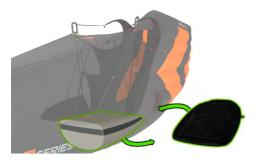
Remove the foam protector and insert the inflatable one with the information sticker facing forward.
