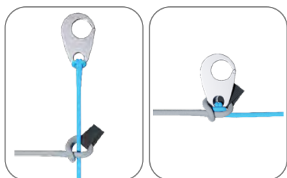
Diagram 1. Speed-bar connection by means of the Brummel hook.
