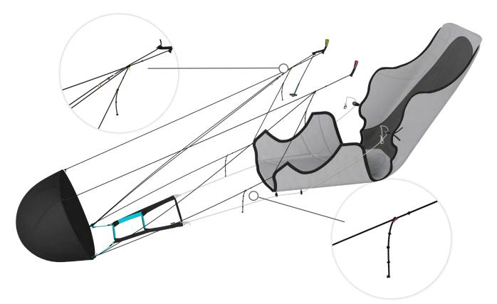
The pod can be adjusted to fit the size of the pilot's legs thanks to the cords situated at the side of the inside of the pod. It is essential that the pod is correctly adjusted so that the pilot is comfortable during flight. Adjust it in a hang frame before your first flight. Niviuk R+D pilots provide the following tip for getting into the pod without getting stuck: put your left leg in first, and then put your right leg in. Using the straps, adjust it to your individual preference.
